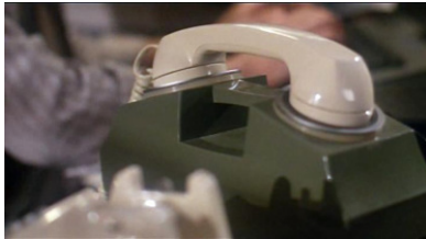
Figure 1: The acoustic coupler in WarGames
