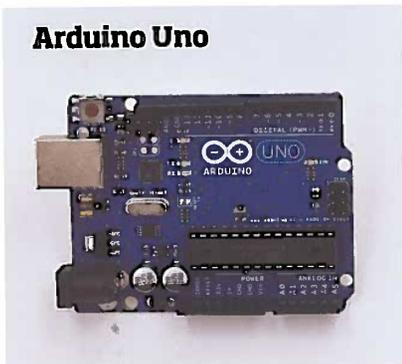
The Arduino Uno microcontroller is inexpensive, open source, beginner-friendly, and has a huge code base to help you get started making gadgets fast. An awesome tool for physical computing, the Arduino platform consists of a microcontroller board, plus the free Arduino software development environment.
